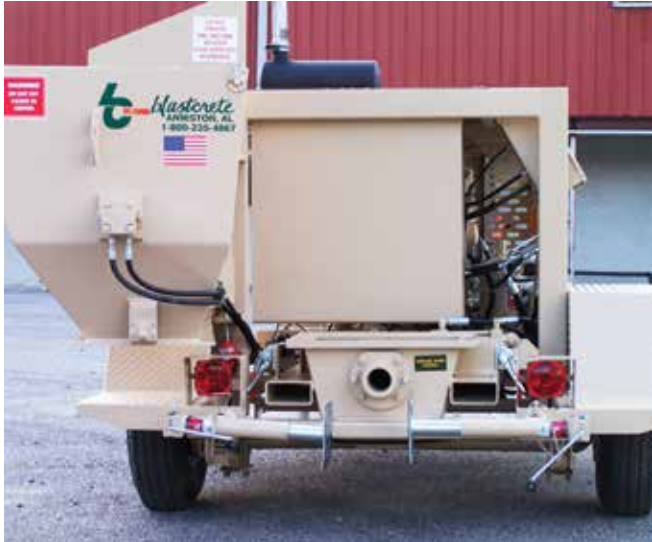
Swing-out hoppers give users easy access to the pump kit for maintenance
