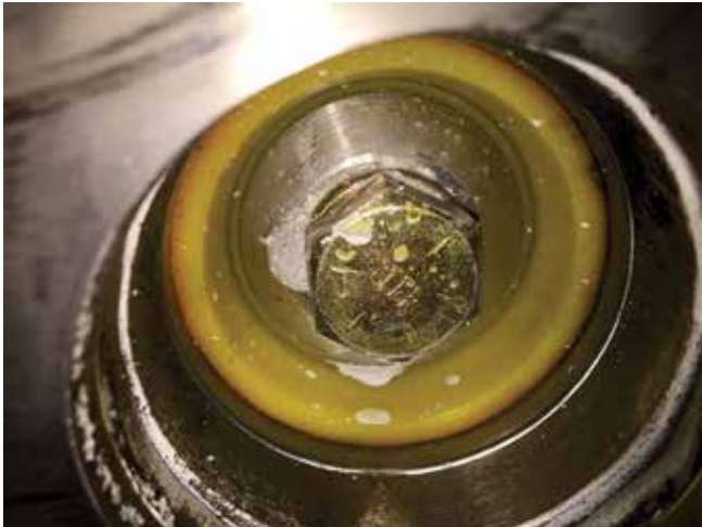
Cup seals, or piston cups, attach to the end of the hydraulic rams and are the most common wear parts on swing tube piston pumps
