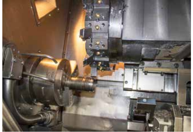
Fig. 8: A CNC-controlled lathe machines a shotcrete nozzle body. This lathe has eight tools in its magazine and can load steel blanks and unload finished parts automatically. Normally, the part would be covered in a stream coolant during machining. This nozzle body begins as a piece of steel tubing and has all its features machined into it. Additionally, these nozzle bodies are case-hardened after machining (Photo courtesy of Construction Forms, Inc.)
