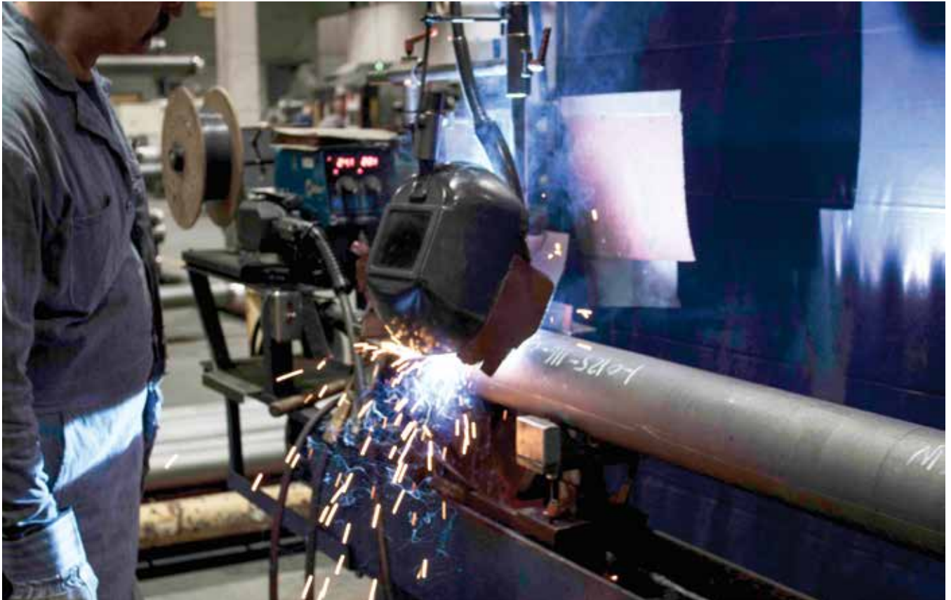
Fig. 4: The raised flange end is welded onto cut-to-length tubing. This machine is semi-automated and welds both ends of the pipe simultaneously. Depending on the size and shape of the parts, some are welded by more automated robotic welders and some parts are welded by hand. Many different combinations of weld type (for example, TIG, MIG), weld wire, technique, and machine settings are used on different types of products (Photo courtesy of Construction Forms, Inc.)
