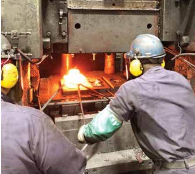
Fig. 7: A forge employee positions a hot steel blank to be formed into shape on a forging press capable of pressing with 2500 tons (3.3 million kg) of force. The press is several stories tall, reaching above and below ground. There are three progressive shapes in this die set; the blank will be moved from one impression to the next each time the press closes (Photo courtesy of Cornell Forge Company)
