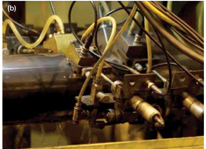
Fig. 2(a) and 2(b): A continuous ribbon of steel, up to 11/16 in. (17 mm) thick at this mill, is unrolled and fed into the tube welding mill. Rollers progressively curl the sheet into a tube. Induction coils heat the edges of the ribbon and rollers press the edges together to the final tubing diameter, creating a weld seam. Sensors monitor weld seam quality immediately after the tubing is welded (Photos courtesy of ArcelorMittal Shelby)
