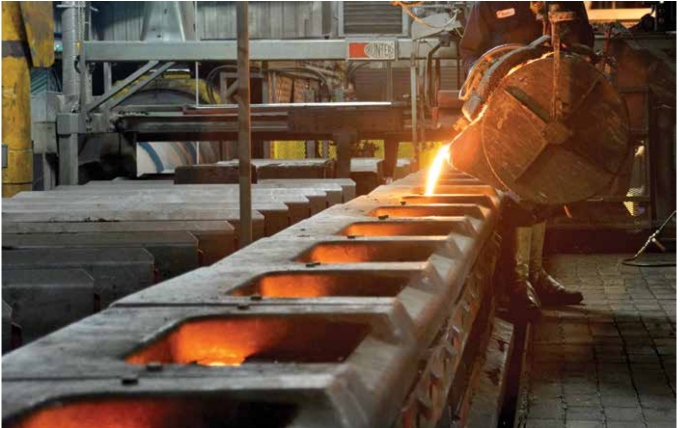
Fig. 6: A foundry employee pours molten iron into sand molds on this semi-automated production line. This machine will typically produce a mold every 1 to 2 minutes. Each mold may have several cavities, producing several pieces of a part with each pour. A large weight is set on the top of each mold to keep the top half of the mold from floating up on the molten metal (Photo courtesy of Alliant Castings)
