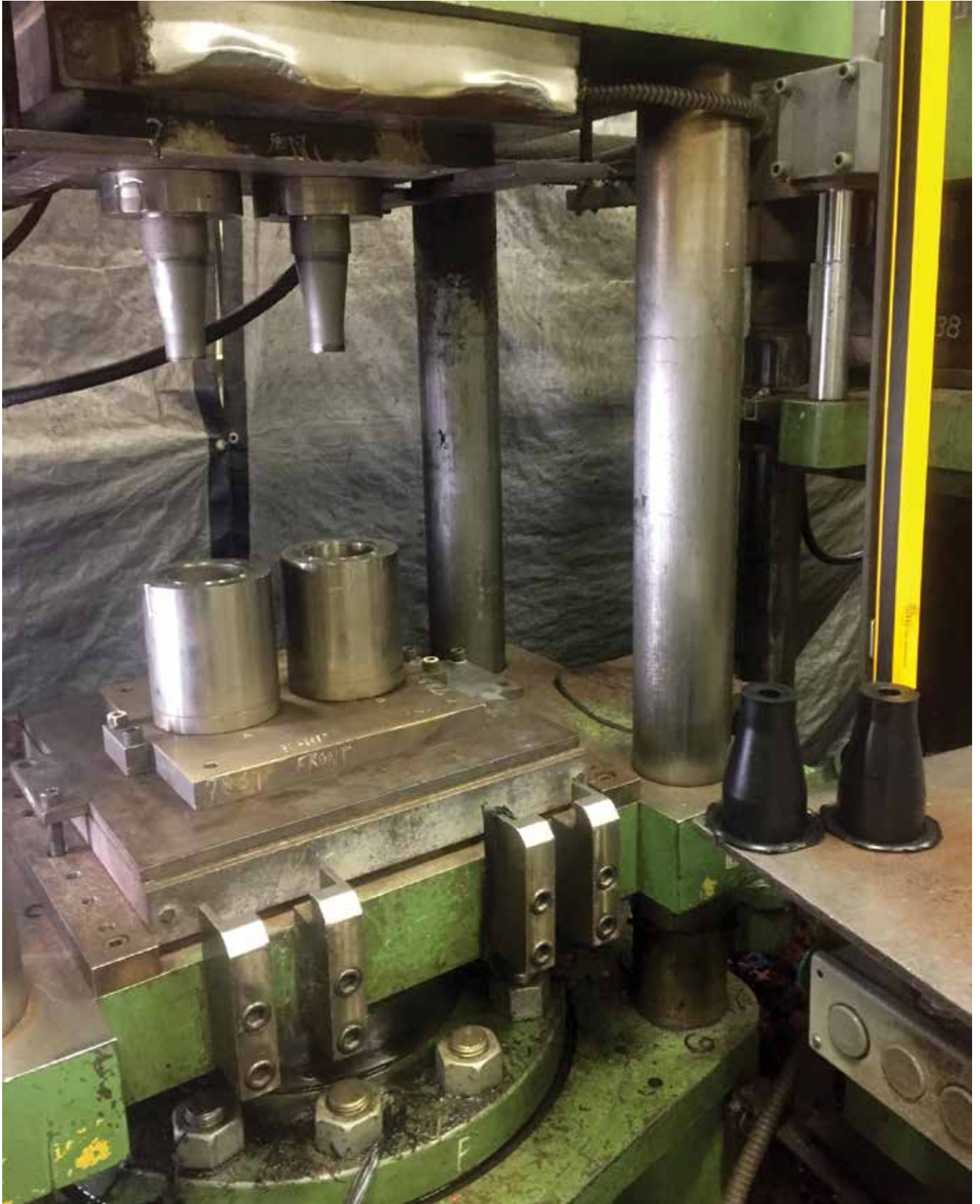
Fig. 9: Rubber nozzle tips are produced by compressing a rubber block or injecting rubber into a mold. The rubber is heated and cured while in the mold, setting the final shape and properties (Photo courtesy of Molded Dimensions Inc.)
