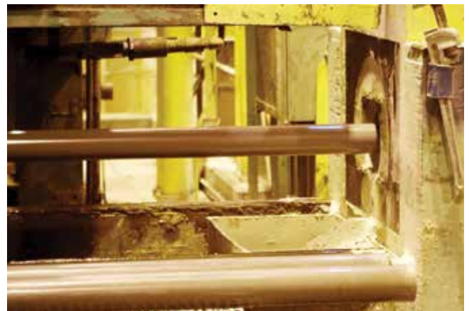
Fig. 3: Tubing is pulled over a mandrel and through a die set. At this mill, powerful electric motors can pull the tubing with up to 1,000,000 lb (450,000 kg) of force. The drawing process thins the tubing wall and reduces the diameter, allowing for precise control of inside and outside diameters. This tubing is known as drawn over mandrel (DOM) or cold drawn tubing (Photo courtesy of ArcelorMittal Shelby)
