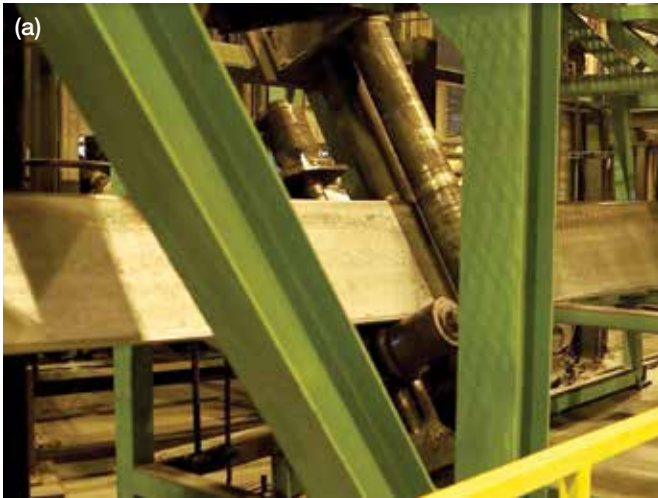
Fig. 2(a) and 2(b): A continuous ribbon of steel, up to 11/16 in. (17 mm) thick at this mill, is unrolled and fed into the tube welding mill. Rollers progressively curl the sheet into a tube. Induction coils heat the edges of the ribbon and rollers press the edges together to the final tubing diameter, creating a weld seam. Sensors monitor weld seam quality immediately after the tubing is welded (Photos courtesy of ArcelorMittal Shelby)
