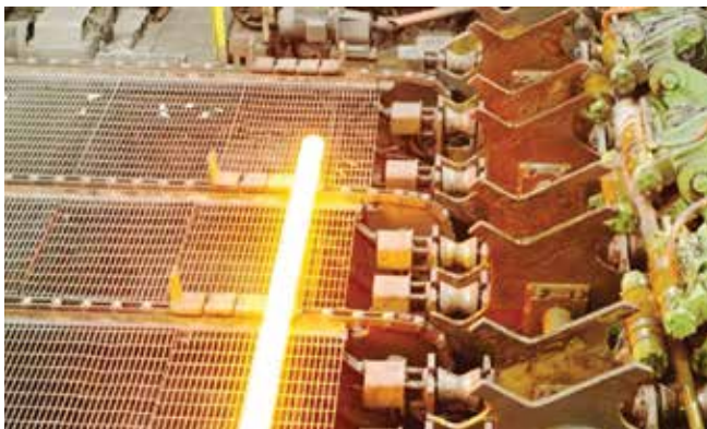
Fig. 1: A newly formed seamless steel tube rolls out of the seamless mill. The stabilizing rollers and piercing bar can be seen on the right. The solid billet, heated to 2250°F (1230°C), is forced in at the top right while being pressed and rotated. The tubing rotates, being pressed and stressed by the piercing rollers, while the piercing bar opens the inside diameter (Photo courtesy of ArcelorMittal Shelby)
