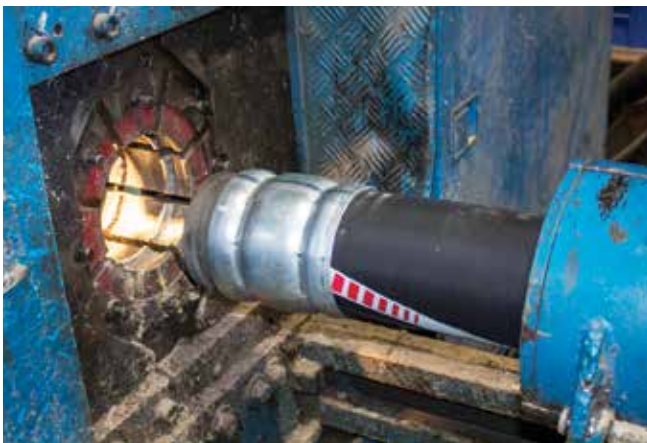
Fig. 5: A powerful crimping press inserts the hose barb into the hose, then compresses the ferrule onto the hose, securing the hose barb in place. This press is hydraulically powered and has eight dies that close simultaneously around the ferrule (Photo courtesy of Construction Forms, Inc.)
