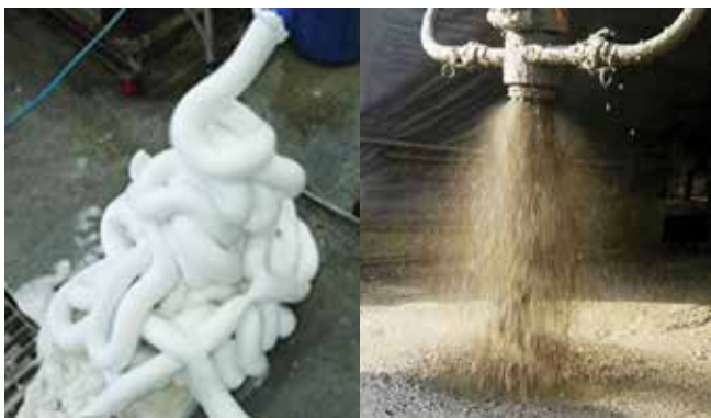
Fig. 1: (a) Cellular material; and (b) spraying cellular sprayed concrete
