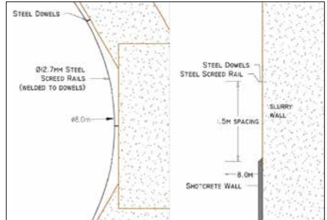
Fig. 5: Screed rail setup
