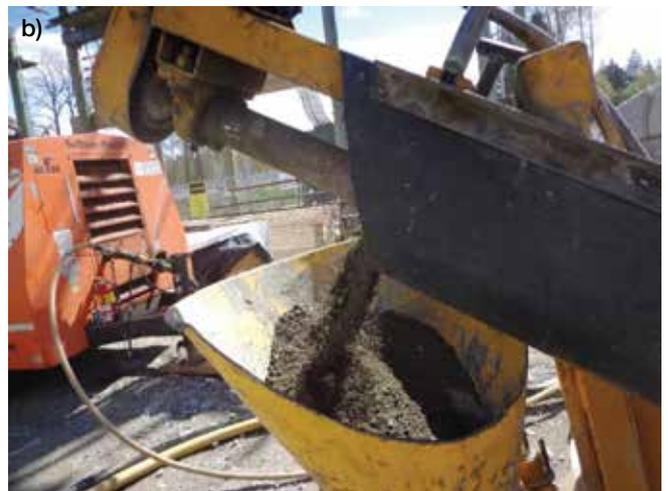
Fig. 13(a) and (b): Dry-mix shotcrete machine with predampener
