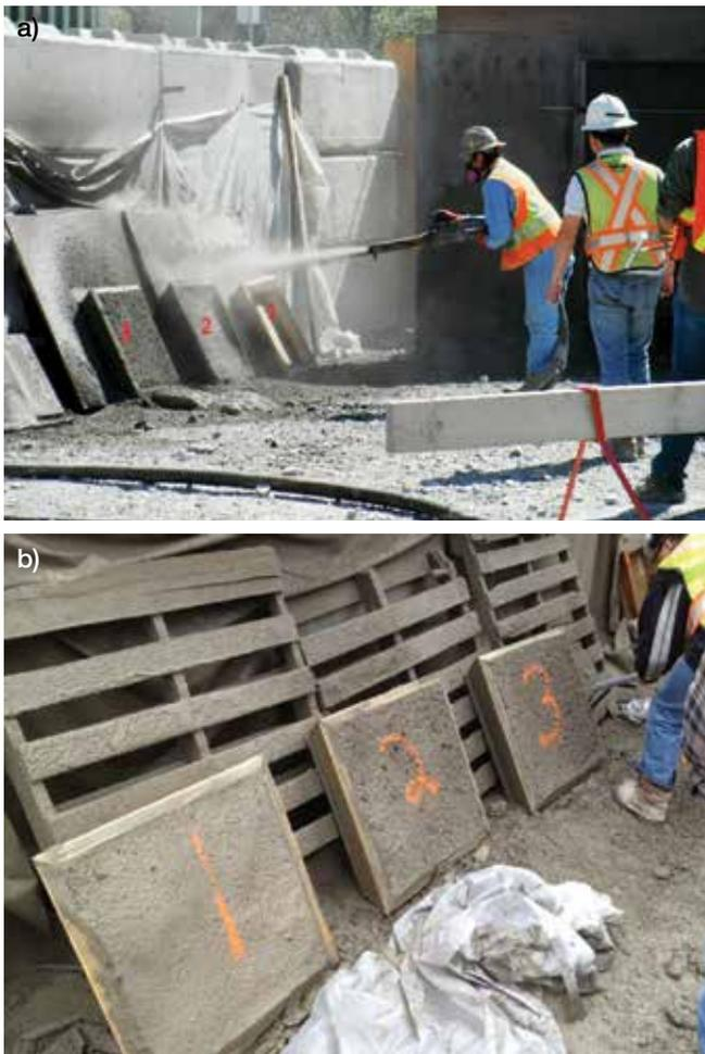
Fig. 9: Nozzlemen qualification: (a) shooting test panels; and (b) setting time and early strength tested for each mixture
