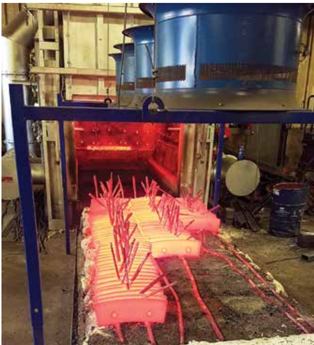
Fig. 6: Heat-treat oven—a load of castings is pulled out of the batch heat treating oven. This alloy is quenched with forced air, not a water or oil bath. They are positioned below powerful fans, which will blow air over the castings, cooling them rapidly. The pieces of reinforcing bars are used to keep the castings from contacting one another, which would result in uneven heating and cooling (Photo courtesy of Alliant Castings)
