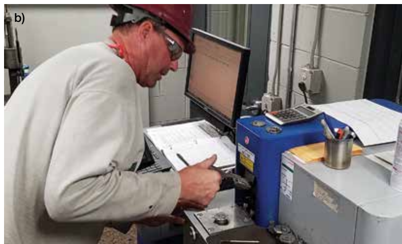
Fig. 1: Chemistry sampling: (a) taking a sample—a furnace operator takes a sample of molten metal from the furnace. He will pour the metal into a water-cooled mold to quickly make a sample for the quality control laboratory; and (b) spectrometer—a technician places the metal sample cylinder, or button, on the sample stage of the spectrometer. This machine will analyze the chemistry of the metal in just seconds, allowing the technician to approve the chemistry of the sample or inform the furnace operator how much alloying elements to add to this melt (batch) of metal
