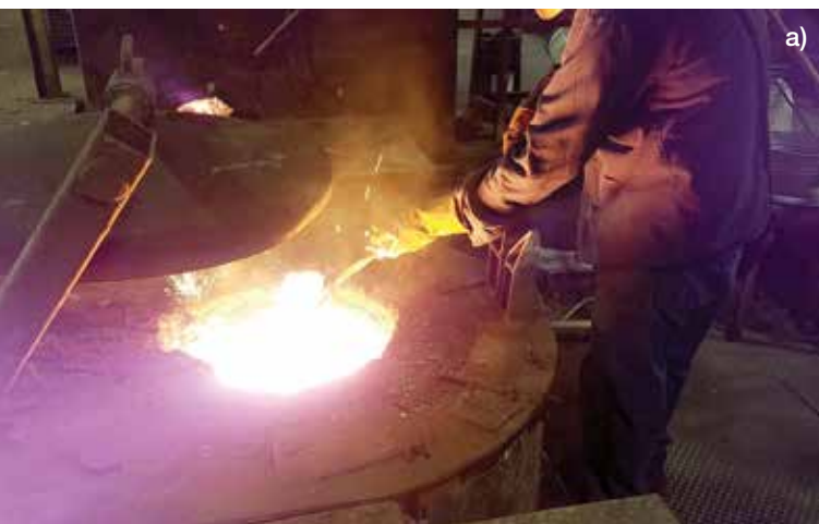
Fig. 1: Chemistry sampling: (a) taking a sample—a furnace operator takes a sample of molten metal from the furnace. He will pour the metal into a water-cooled mold to quickly make a sample for the quality control laboratory; and (b) spectrometer—a technician places the metal sample cylinder, or button, on the sample stage of the spectrometer. This machine will analyze the chemistry of the metal in just seconds, allowing the technician to approve the chemistry of the sample or inform the furnace operator how much alloying elements to add to this melt (batch) of metal
