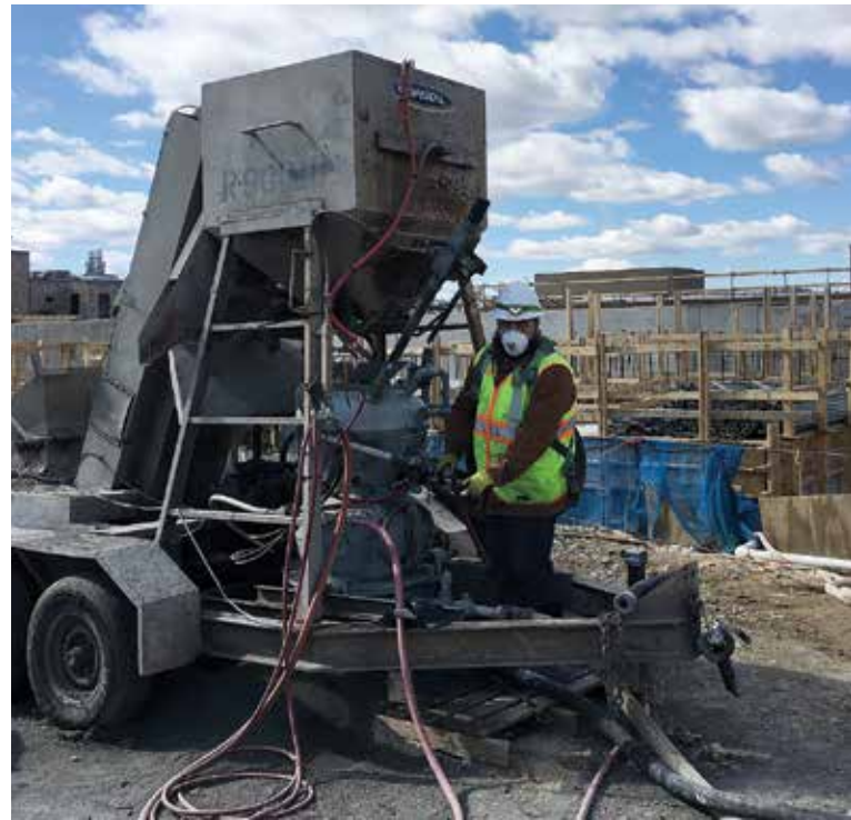
Fig. 2: N-style gun and mixer rig
