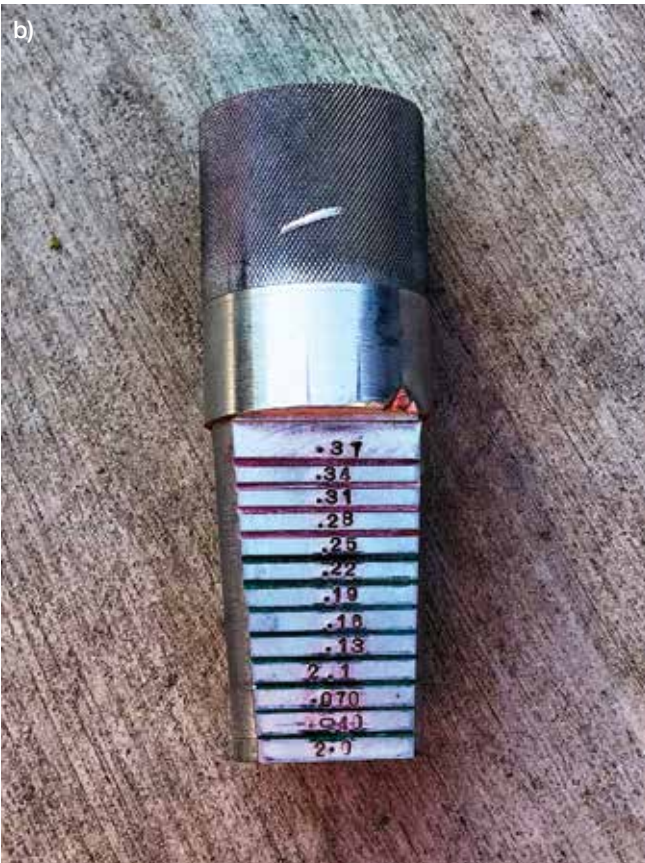
Fig. 1(a) and (b): Gauge to measure wear levels
