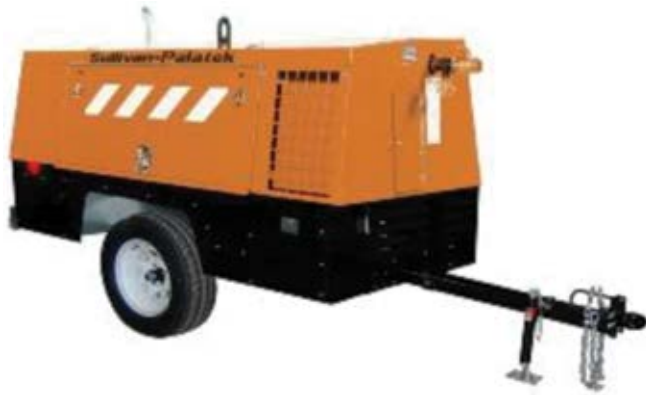
Fig 2: Although nice and clean outside, poorly maintained components may significantly reduce available air flow
