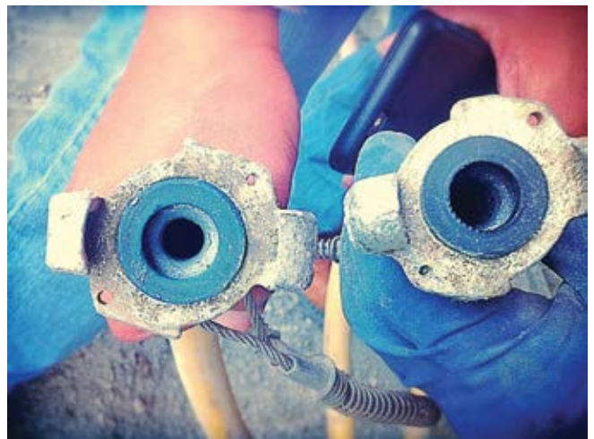
Fig. 4: Although identical in exterior appearance, non-full-flow couplers (left) can be easily identified by their restrictive interior diameter
