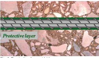
Fig. 1: Passivation (iron oxide) layer
