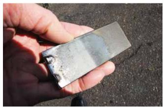
Fig. 3: Same metal plate after being halfway submersed in a high-alkaline (high-pH) water for 24 hours showing the formation of an iron oxide passivation layer (grayish-black)
