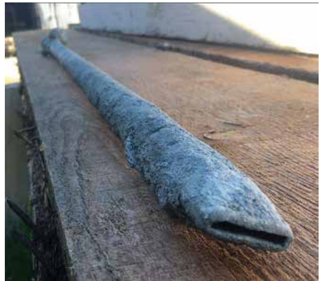
Fig. 6—This blow pipe is constructed from 0.75 in. (19 mm) steel pipe, approximately 3 ft (0.9 m) long. The tip has been shaped to a width of 0.25 in. (6 mm) with common tools to provide a wide fan pattern. It is efficient, durable, and requires very little air
