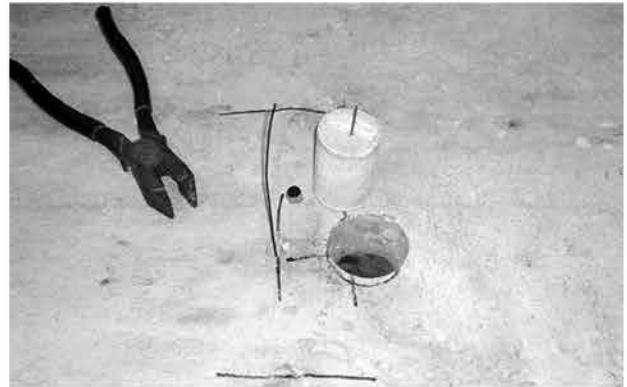
Fig. 11—Secondary hole with reinforcing steel connection.
