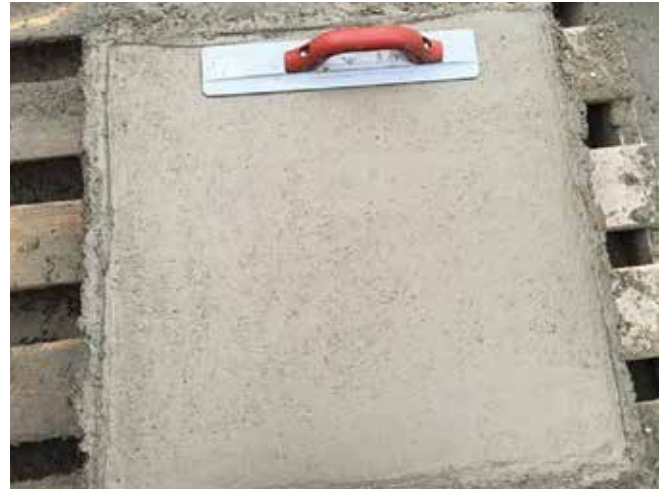
Fig. 11: Natural fiber mixture (WNF) finished with a magnesium trowel
