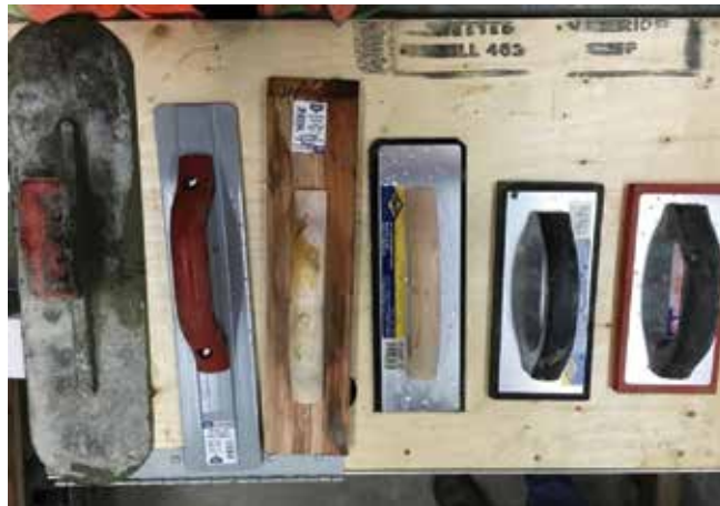
Fig. 9: Finishing tools used, from left to right: steel trowel, magnesium trowel, wood float, hard rubber float, textured rubber float, and sponge float
