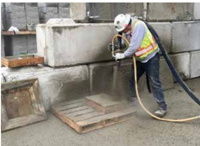
Fig. 4: Shooting into mold for plastic shrinkage cracking testing
