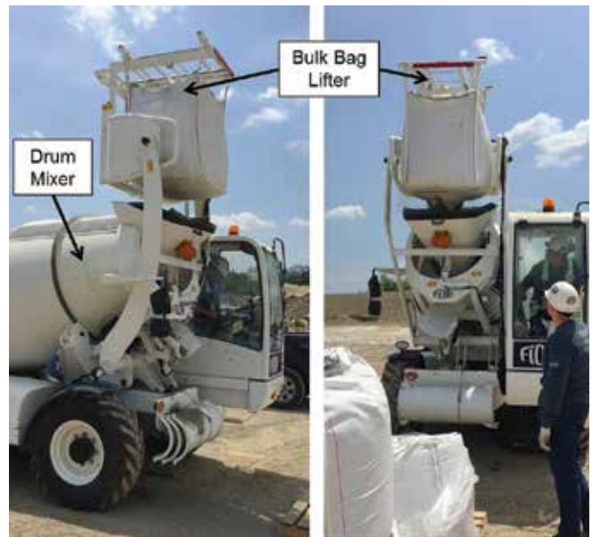
Fig. 5: Mobile self-loading mixer with bulk bag lifter
