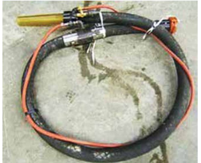
Fig. 10: Hydro-mix nozzle for dry-mix shotcrete (from Hutter, 2014)
