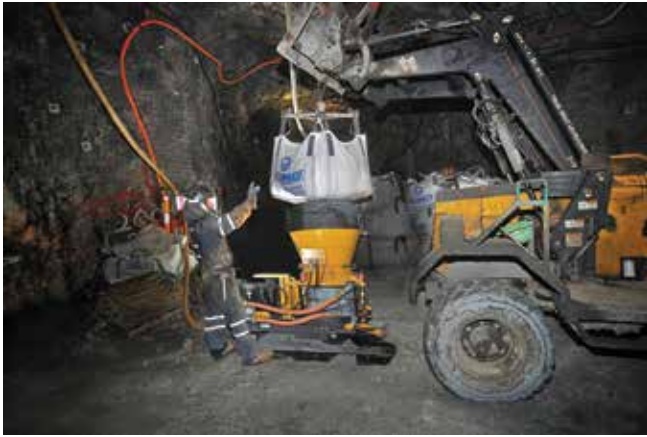
Fig. 8: Bulk pre-packaged tote bag with hopper hood
