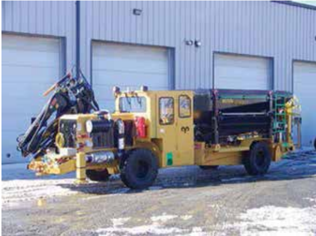
Fig. 6: Bulk dry shotcrete hauler/sprayer
