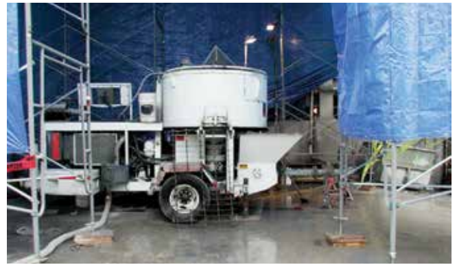
Wet-mix shotcrete pump with a pan mixer for handling bulk sacks works well for mixing and placing large volumes of material
