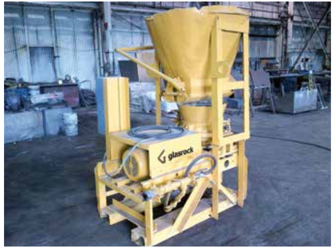
The Jet-Creter was the first straight-drop rotary gun used for refractory installations in the United States. They typically had gasoline engines to run the rotor and were mounted on wheels with a trailer hitch for towing
