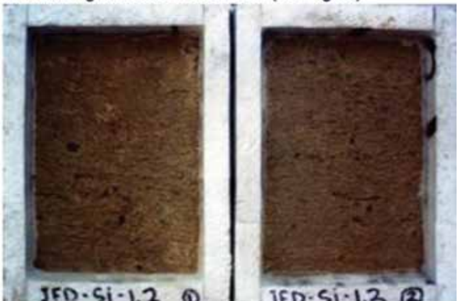
Non-air-entrained versus air-entrained dry-mix shotcrete—air void system, ASTM C457 (60 \times magnification) and salt scaling resistance, ASTM C672
