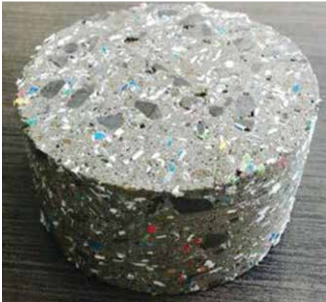
Fig. 7: Shotcrete core containing shredded recycled plastic 14
