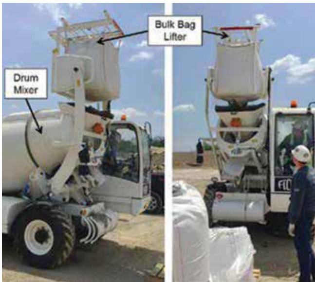
Fig. 4: Mobile concrete mixing unit integrated with a lifting system for bulk, preblended concrete, and shotcrete material bags 10
