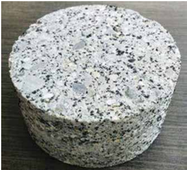
Fig. 8: Shotcrete core containing recycled rubber beads 14
