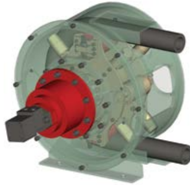
Fig. 2: A squeeze pump operates on the same principal as filling a straw with a milkshake and using your thumb and index finger to squeeze the milkshake out of the straw
