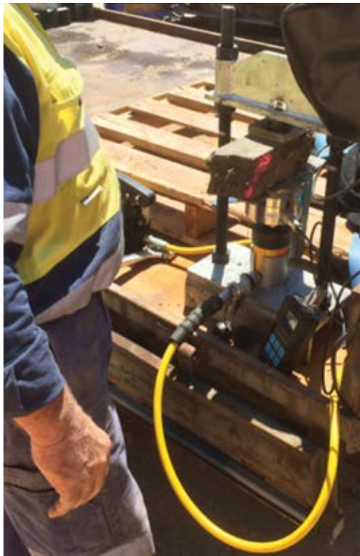
Fig. 1: Setup for beam end test
