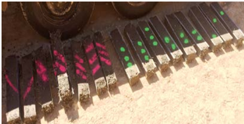
Fig. 2: Beams prepared to test early-age strength development
