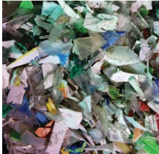
Fig. 3: Plastic aggregates (0.04 to 0.2 in. [1 to 5 mm]) from crushed plastic containers
