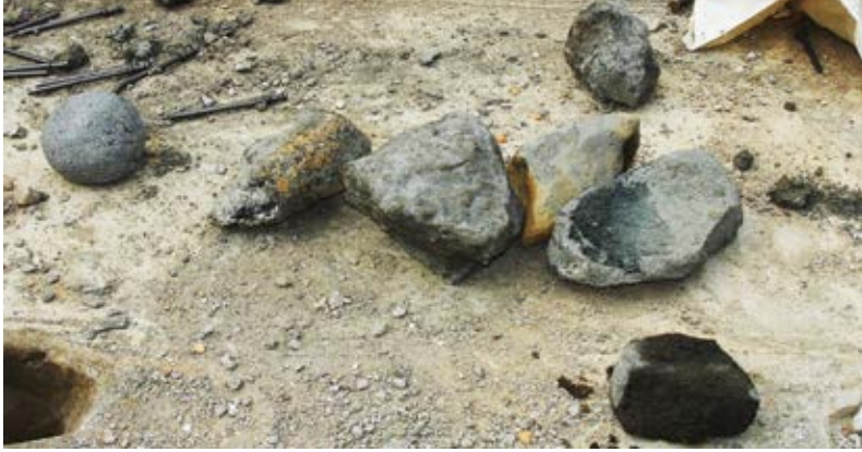
Fig. 4: Large ballast rock caught on the grate. The smaller pieces that managed to slip through the grate caught in the reducer
