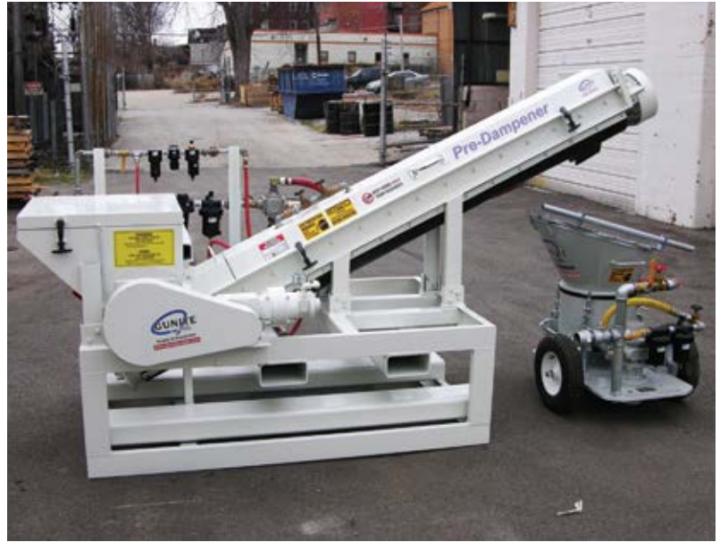
Fig. 2: Predampener shown with dry-mix shotcrete machine
