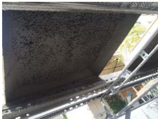
Fig. 1(b): Bond test panel after two layers were shot
