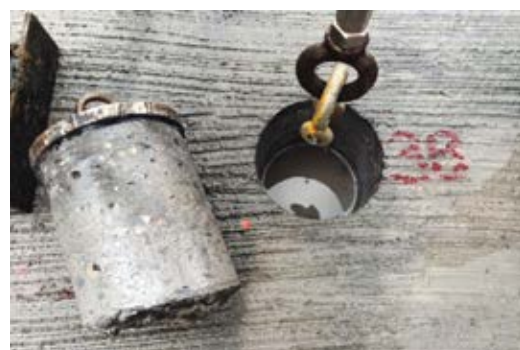
Fig. 5(b): Picture of layer interface failure
