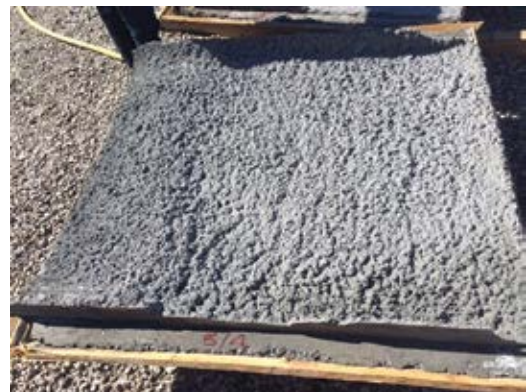
Fig. 2(a): Nozzle-finished panel
