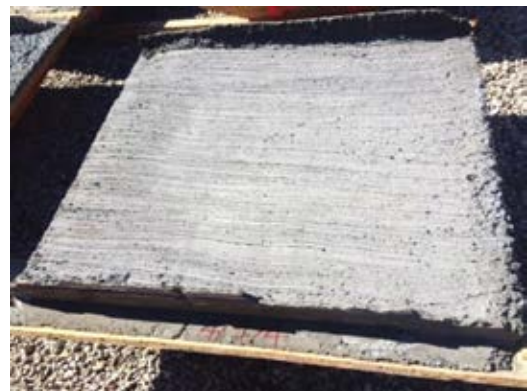
Fig. 2(b): Scratch/etched finished panel, unreinforced
