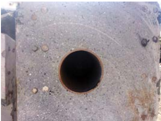
Fig. 7(a): Cut through the single pass wall mockup in layers
