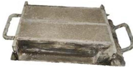
Fig. 4: Steel end-beam mold used for early-age strengths measurements
