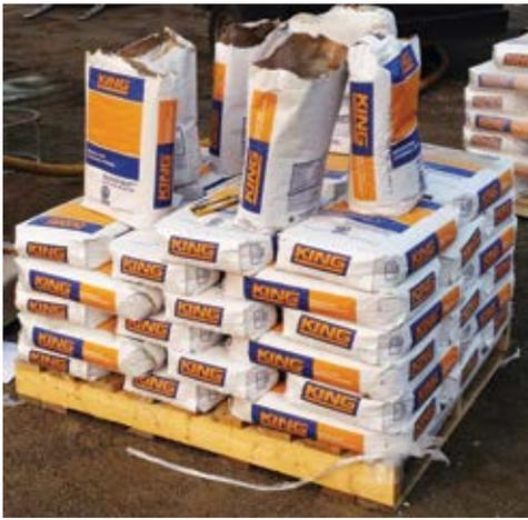
Fig. 1: Candidate shotcrete mixtures packaged in 66 lb (30 kg) bags
