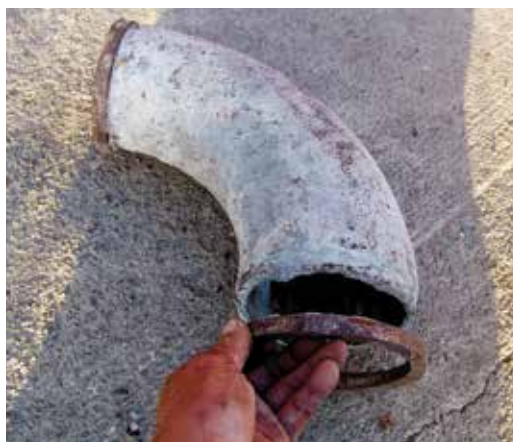
Fig. 4: This elbow failed due to excessive force being transmitted by the pumping system
