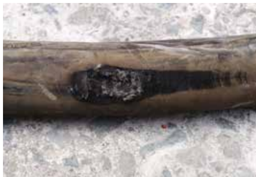
Fig. 3: This hose quickly wore down against a concrete corner and burst
