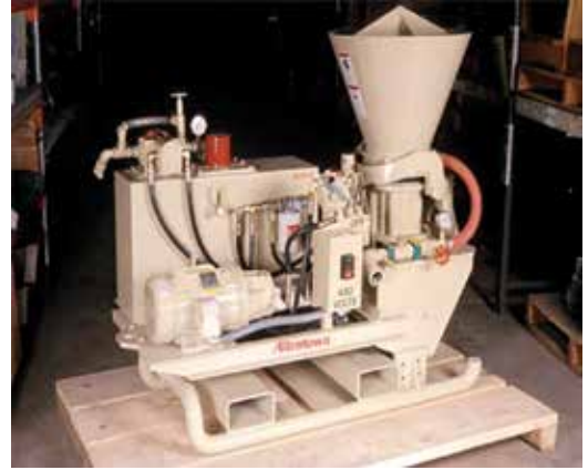
Fig. 5: Rotary guns have over 50 years in the field use. This dry gun barrel-type gun is an air over/hydraulic unit for more consistent material flow and has an external air exhaust to keep it from bubbling up through the hopper during material discharge. This gun type can push macro- and micro-steel and synthetic fibers through the gun. These guns have pushed material over 400 ft (120 m) vertically and over 2500 ft (760 m) horizontally
