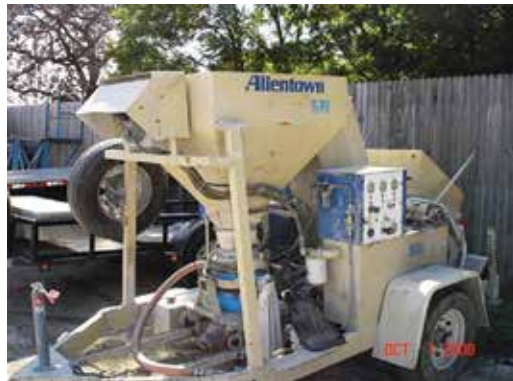
Fig. 10: From the original design this rig is a shorter version of the original predampener and mixing rig with a rotary barrel-type gun and hydraulic water booster pump designed to fit into low spaces, such as parking garages. This rig can mix moist sand and cement or predampen prebagged material
