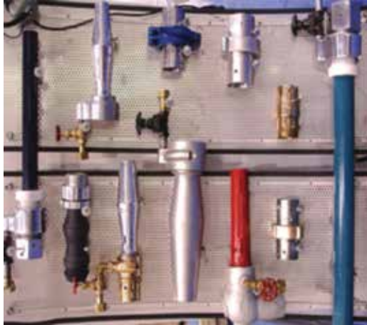
Fig. 4: These dry-process nozzles are designed to handle the high material velocity and produce adequate spray patterns; also shown are different hose coupling sets. Six of the nozzle setups have water rings with 8 to 16 small 1/16 in. (1.6 mm) holes that create a cone when the water is turned on; as the material passes through the water, the material is partially mixed as the nozzleman builds up the layers. The 2 in. (50 mm) setup water ring has 16 straight holes in it and requires more water pressure and air volume to properly mix and compact the material
