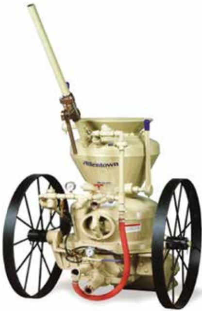
Fig. 7: N-gun or pressure vessel has 105 years of field use. It is based off the original gun design from 1907-1910 and is called the double tank or chamber. This gun allows the material to continuously flow because the bottom chamber stays fully pressurized while the top chamber is being filled. With very few wear parts, these guns are built to last forever. The pressure is still used for pushing material 500 ft (150 m) vertically and 1000 ft (300 m) horizontally
