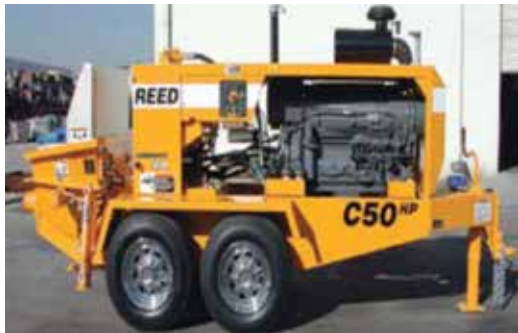
Fig. 13: Reed C50HP concrete pump can be reduced down to a 2 in. (50 mm) hose for shotcrete work or up to a 5 in. (125 mm) hose for concrete pumping
