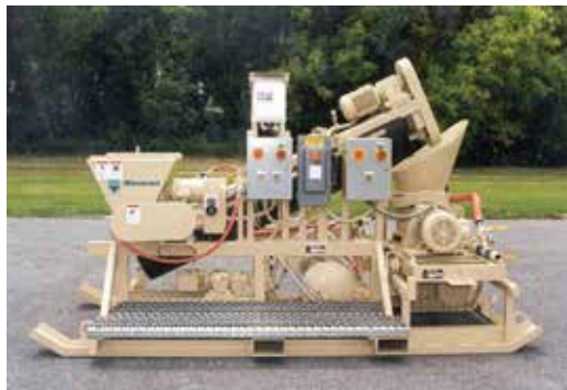
Fig. 8: This auger-feed predampener and rotary barrel gun combination is used in civil tunnels and mining projects. This is an electric feed machine for consistent material flow, along with a peristaltic accelerator dosing pump that injects the metered liquid into the water line to the nozzle for early set times of the in-place dry shotcrete material
