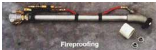
Fig. 1: Fireproofing nozzle setup
