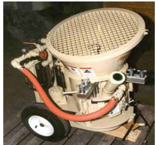
Fig. 6: Bowl guns have been used over 50 years in the field use. It has no external exhaust, allowing the excess air to bubble up through the hopper. The U-shaped bowl makes it difficult to push macro-synthetic and steel fiber mixtures up and through the material outlet and limits the horizontal distance the material can be pushed
