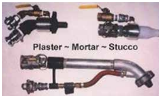
Fig. 2: Plastering nozzle setups
