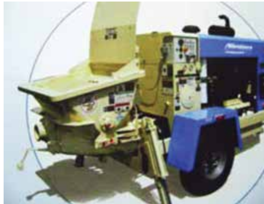
Fig. 15: Allentown Powercreter Model 40 pump with hydraulic outriggers can be reduced down to a 2 in. (50 mm) hose for shotcrete work or up to 5 in. (125 mm) for concrete pumping. The electronic swing tube control allows for faster shifts between cylinders, thus reducing the line surge to the nozzleman
