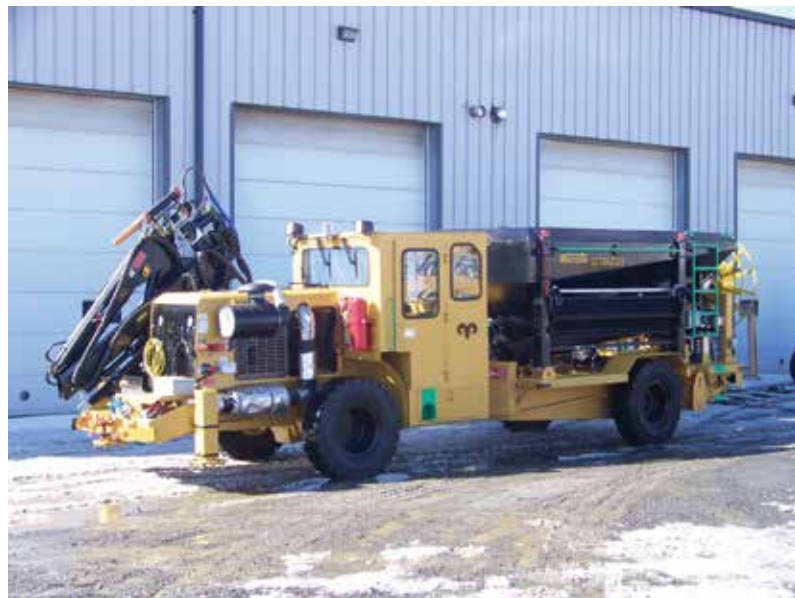
Fig. 1: Bulk dry shotcrete hauler/sprayer
