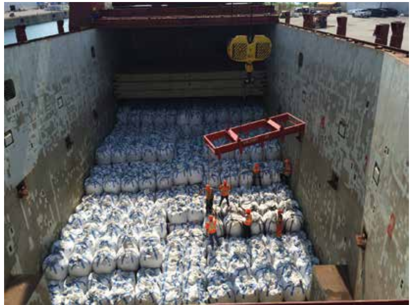
Fig. 2: Preblended dry shotcrete being loaded into a ship's hull
