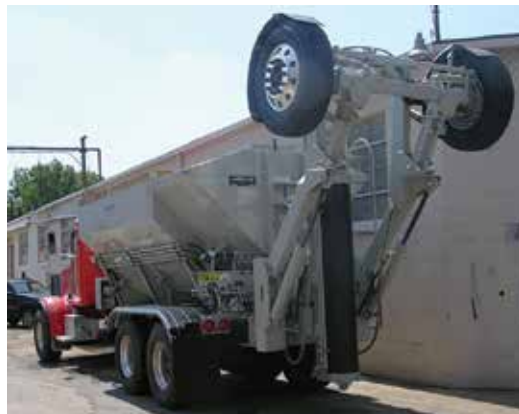
Fig. 1: On-site dry-mix batching truck
