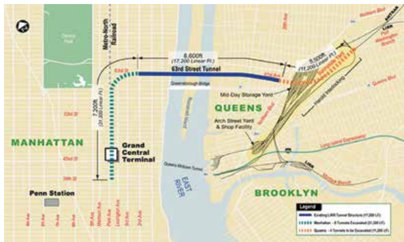
Fig. 1: East Side Access overall project scope
