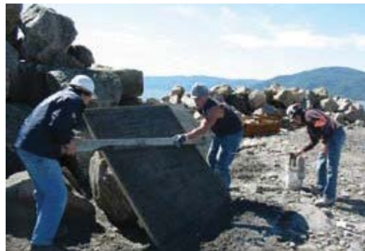
Test panels were shot to evaluate the competence of the nozzlemen and to confirm hardened properties of the mixture
