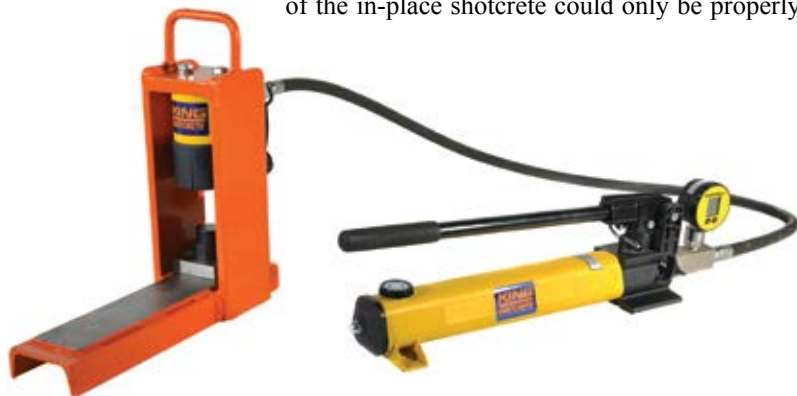
Fig. 4: The end beam tester provided one mine with the information required to change their procedures so that the stope could be filled just 24 hours after placement, translating into a full day's reduction in cycle time
