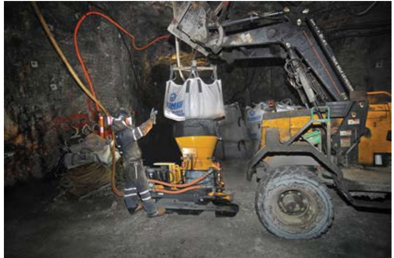
Fig. 2: When using bulk tote bags, a hopper hood manufactured to fit the hopper of the shotcrete machine will seal the hopper and prevent dust from being released
