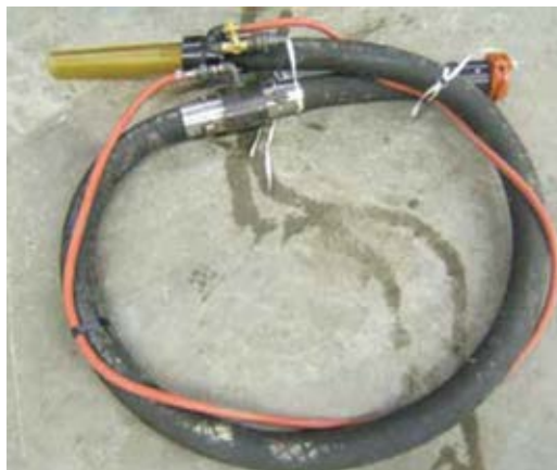
Fig. 4: A hydromix-nozzle or semi-wet nozzle (one in which the water ring is moved back several feet from the nozzle) will also prevent the dust generation at the nozzle
