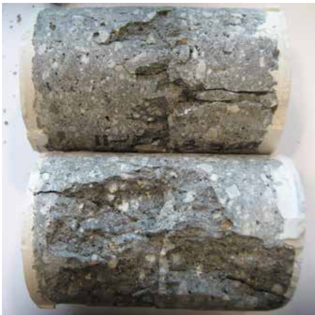
Fig. 7: Low-strength shotcrete cores from one nozzleman, with overspray in the middle
