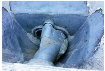
*Fig. 1: Missing auger cannot provide adequate cylinder filling. Uneven nozzle flow will affect nozzle placement quality*
