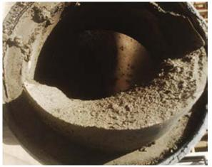
*Fig. 3(c): Hardened buildup restriction inside the S tube is caused by worn wear components*
