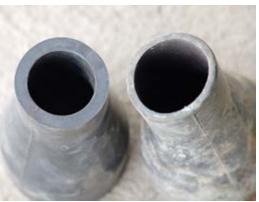
Fig. 6: Worn tip (right)
