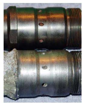
*Fig. 4: Note plugged air ring port on lower nozzle. A single plugged port will dramatically reduce in-place compaction/consolidation quality*
