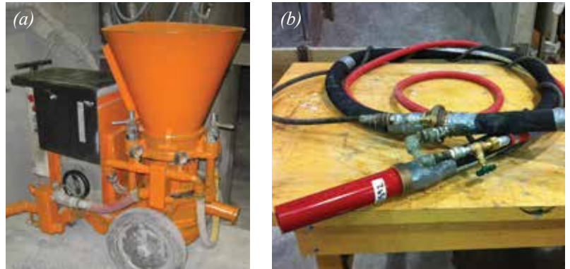
Fig. 2: (a) Spraying gun; and (b) hydromix nozzle
