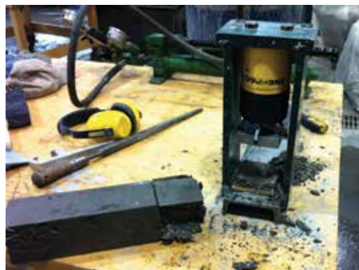
Fig. 4: End beam test apparatus
