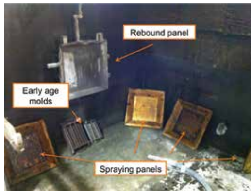
Fig. 5: Rebound chamber before spraying
