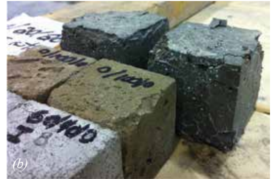
Fig. 7: (a) Expansion of a mixture close to the expansion line; and (b) expansive mixture compare to a stable mixture
