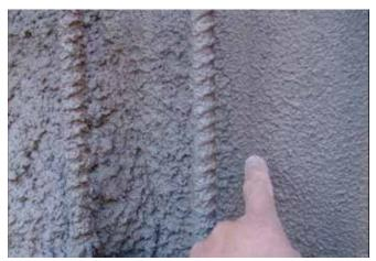
Fig. 3: Note fine materials developing a paste layer at leading edge of the nozzle spray pattern. Although larger particles have impacted this area, they cannot embed until a sufficiently thick paste layer develops
