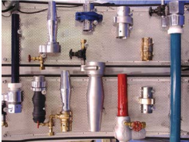
The dry-mix process nozzles are designed to handle the high material velocity and produce adequate spray patterns
