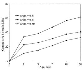
Fig. 4: Development of compressive strength of concrete with different w/cm (RHA content = 10%) (Originally from Fig. 2-4 of ACI 232.1R-00 [Zhang and Malhotra]) (Note: 1 MPa = 145 psi)
