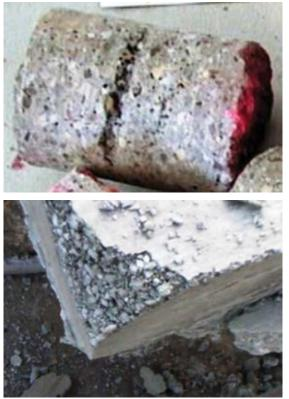
Fig. 1: Poor placement techniques have produced sand lens or encased rebound trapped within test specimen
