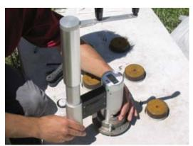
Fig. 4: A pulloff test being conducted on a test panel (photo courtesy of the Centre de recherche sur les infrastructures en béton (CRIB))
