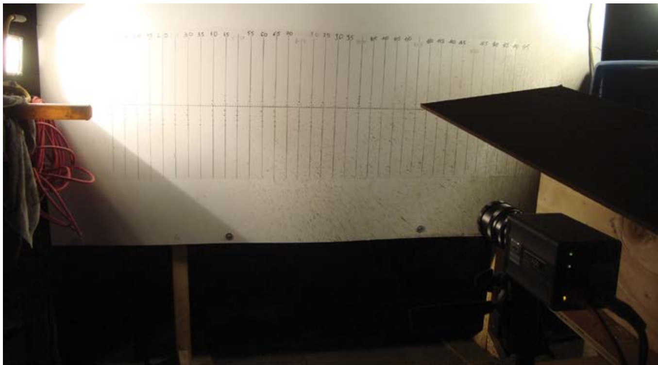
Fig. 3: High-speed camera ready to film a shotcrete spray
