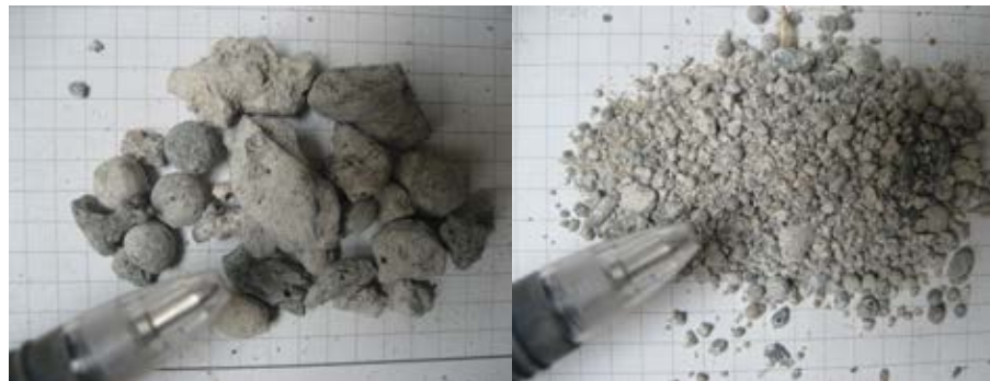
Fig. 1: Pelletized coarse (1.15 to 9.50 mm [0.05 to 0.37 in.]) (right) and pelletized fine (0 to 2.36 mm [0 to 0.09 in.]) (left) blast-furnace slag aggregates
