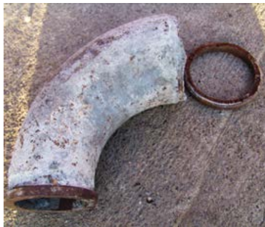
Fig. 1: The importance of safety in the shotcrete world: a 5 x 4 in. (125 x 100 mm) heavy-duty reduce fitting with broken heavy-duty ring
