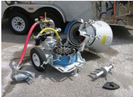
Fig. 5: Gunite machine components
