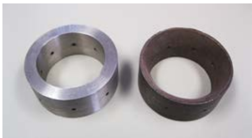
Fig. 6: New water ring (left), worn water ring (right)
