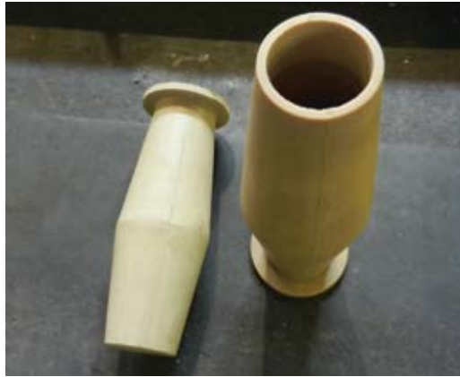
Fig. 8: Dry-mix nozzle liner with interior steps/ridges
