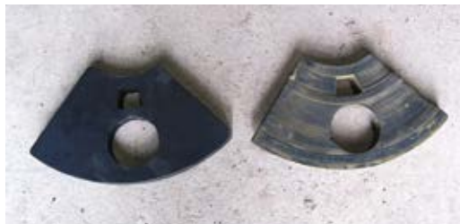
Fig. 4: New wear pad (left), worn wear pad (right)
