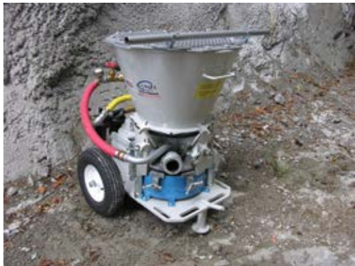
Fig. 1: Bowl-type rotary gunite machine (dry-mix shotcrete machine)
