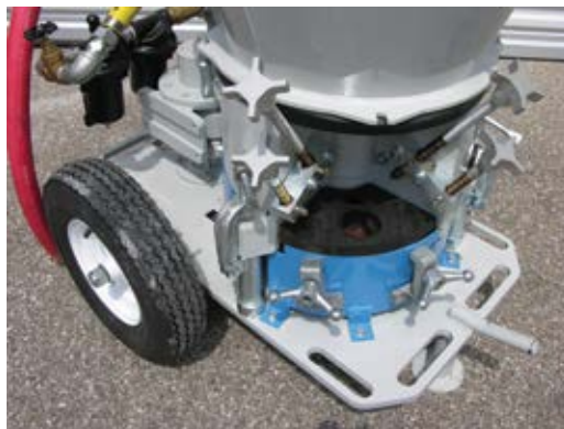
Fig. 3: Gunite machine view of wear pad
