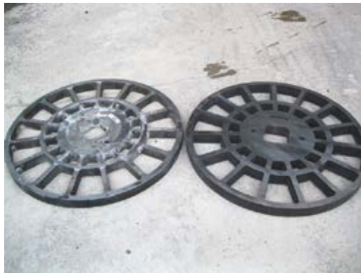
Fig. 2: Worn plate (left), new plate (right)
