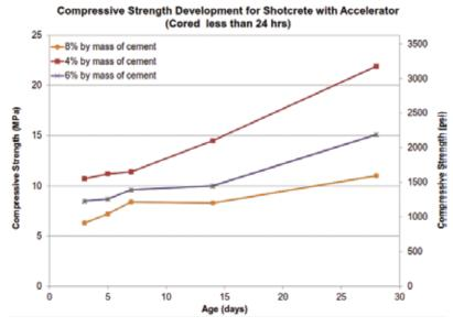
*Fig. 1: Compressive strength development for shotcrete with accelerators; cores extracted at less than 24 hours of age*
