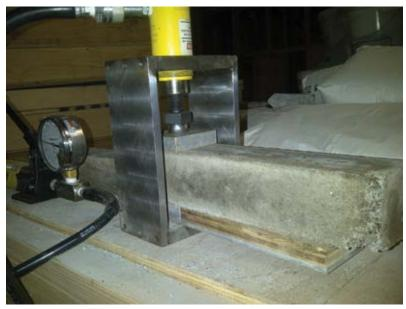
*Fig. 3: End beam test equipment to test compressive strength at less than 24 hours*
