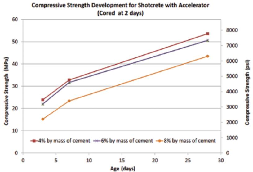
Fig. 2: Compressive strength development for shotcrete; cores taken at 2 days of age
