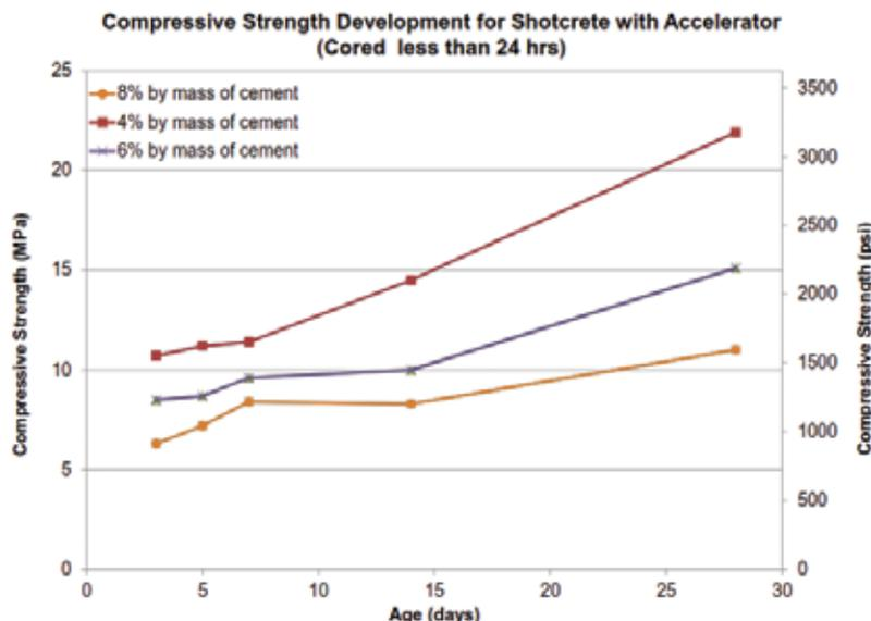
Fig. 1: Compressive strength development for shotcrete with accelerators; cores extracted at less than 24 hours of age
