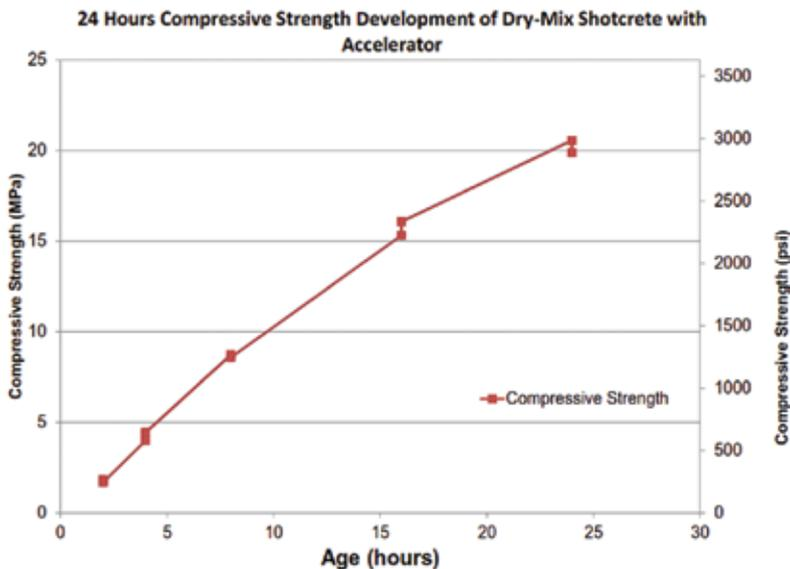
Fig. 4: Early-age compressive strength when tested with end beam tester
