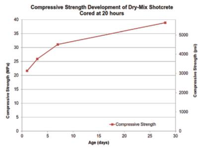
*Fig. 5: Compressive strength development through 28 days; cores extracted at 20 hours*
