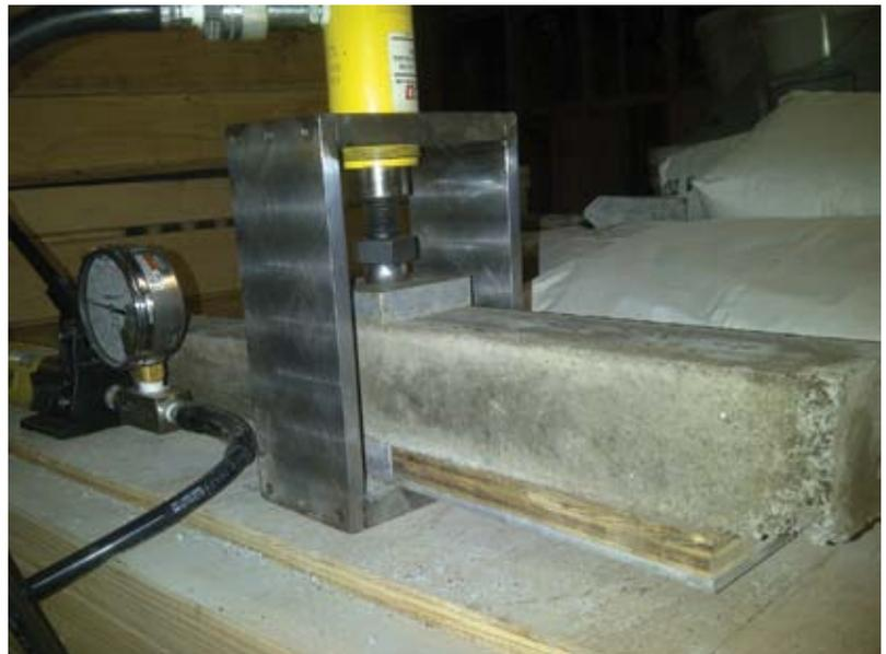
Fig. 3: End beam test equipment to test compressive strength at less than 24 hours
