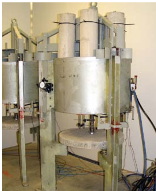
Fig. 2: One of the four creep rigs used for gravity-load testing of specimens
