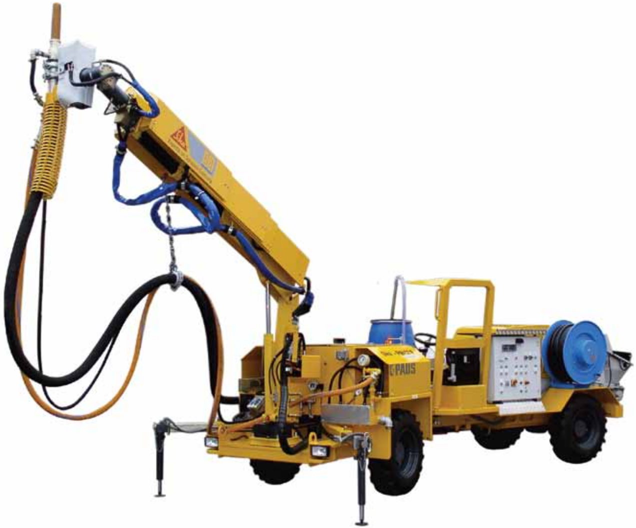
Shotcrete spray arms can reach heights ranging from 10 ft (3 m) to over 72 ft (22 m) and are operated via remote control
