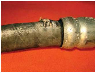
Fig. 2(a): This nearly new hose has burst within days of being run over by equipment. Note the lack of external evidence of internal abrasion damage, as seen in Fig. 2(b)
