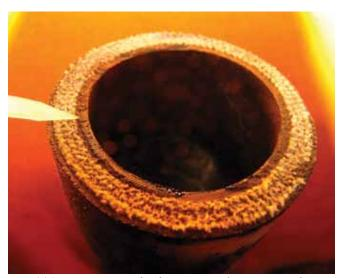
Fig. 1(a): Hose section displaying inner liner area and braided fabric cords
