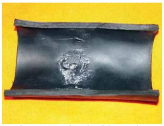
Fig. 1(b): Interior view of inner liner failure caused by crushing
