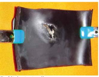
Fig. 2(b): Interior view of burst area
