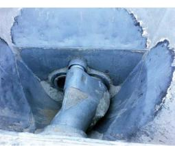
Fig. 2: A wet-mix pump with missing auger cannot effectively fill material cylinders. Unpredictable flow and slugging will affect nozzleman placement quality
