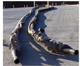
Fig. 1: Although visibly similar, nozzle end hoses may feel very different to a nozzleman. Choose an end hose that is sufficiently rigid, not "doughy"
