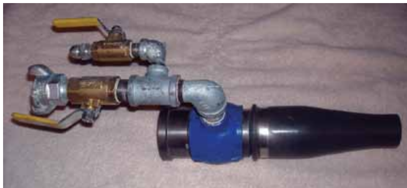
Fig. 2: ACME nozzle with integrated air/accelerator port
