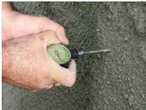
Fig. 3: Pocket penetrometer test
