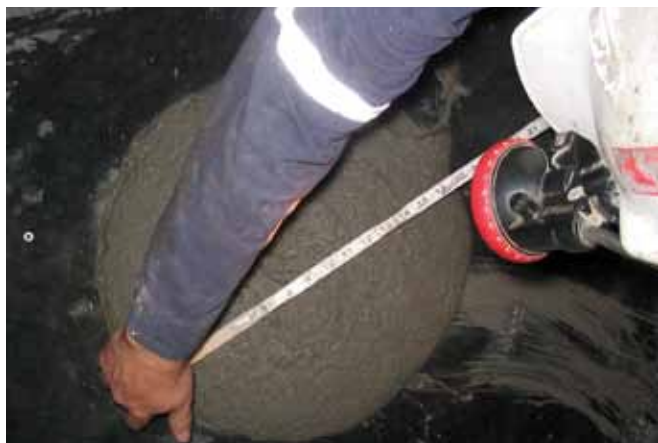
Mining technician measuring the slump flow of a shotcrete mixture
