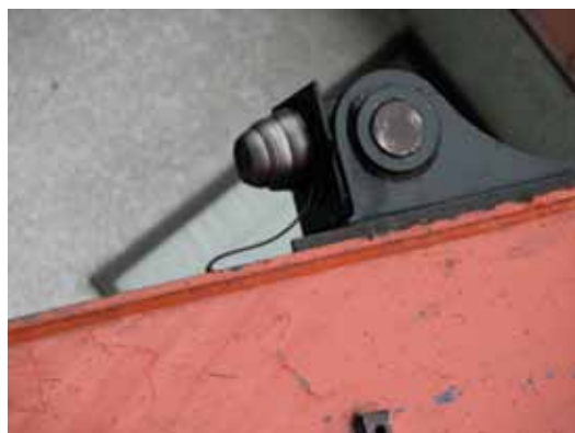
Fig. 12: Camera to assist operator’s vision of bucket
