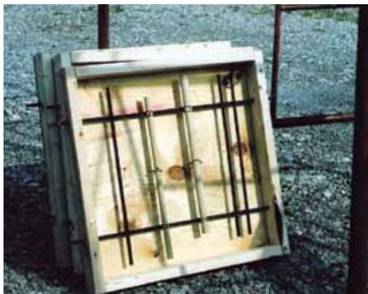
A shotcrete panel form with the simulated reinforcing bars
